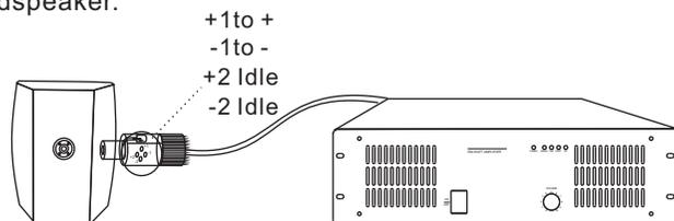
After well connected, please lower the amplifier volume to minimum, and then turn on amplifier, select audio source and adjust the volume to suitable level.
